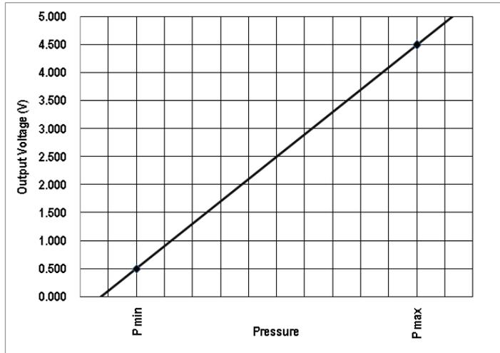
$$\text{Output Voltage} = \left[ \frac{0.8}{(P_{\max} - P_{\min})} \times (\text{Pressure applied} - P_{\min}) + 0.1 \right] \times \text{Supply Voltage}$$
