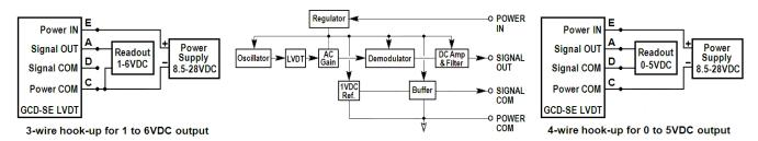
A through E: Connector pin assignments
