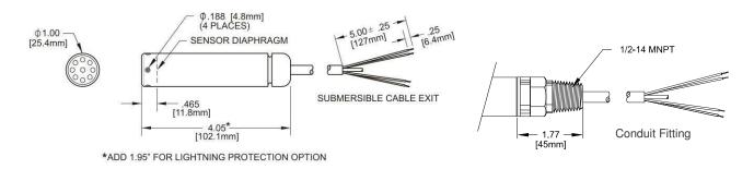
**Gland Cable Seal Configuration for ETFE Cable**
